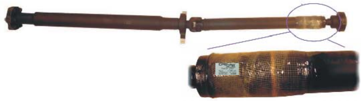
Glass-fiber reinforced epoxy resin for durable use without mechanical damage
